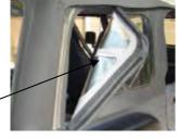
Step (1): Remove the quarter windows and rear window. Remove the metal tailgate bar from the bottom of the rear window and set to the side. It will be reused.
