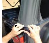
Step (6): Close the header latches to secure the front of the top to the windshield. Catch the hook in the slot in the windshield frame and then close the lever over it so that it lays flat against the windshield frame.
